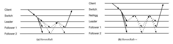
**Figure 5.** The communication patterns in our design resulting from separating replication from ordering and using in-network fan-in/fan-out. Solid arrows refer to application requests and replies. Dotted arrows refer to SMR messages.
