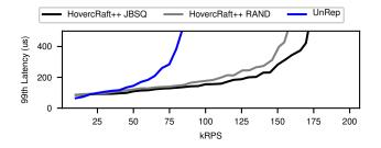
**Figure 11.** Latency versus throughput for a  $S = 10\mu s$  service time with bimodal distribution on a 3-node cluster. Requests are 24-bytes, replies are 8-bytes, and 75% of operations are read-only.
